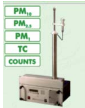
EDM 180 (Grimm) Mass, size distr. 31 ch. Light Scattering (Nephelometer)
