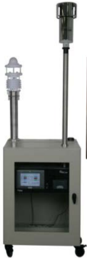
FIDAS (Palas) PNC, Mass (PM 1 , 2.5, 4, 10, TSP) LED light scattering
