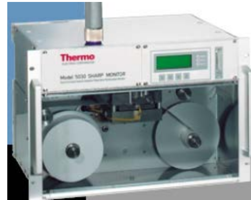
SHARP (Thermo) Mass; Nephelometry + \beta -Absorption
