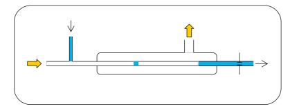
Membrane sampler with electrochemical detection
