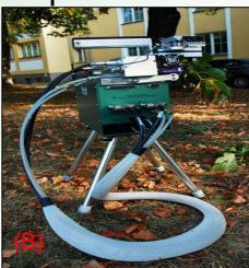
Portable Photosynthesis System LICOR model 6200 (A) and 6400 (B) (Lincoln, Nebraska, USA)
