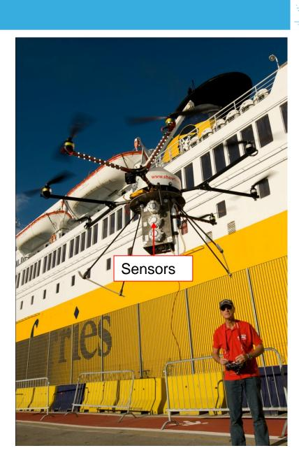
Ship exhaust plume measurement from unmanned flying platform: verification of "ship fuel" directive on sulphur in marine fuel:
