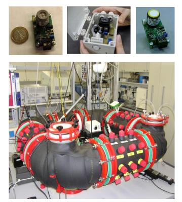
Laboratory testing at controlled wind/temperature/humidity conditions with varying air pollutant and interfering substances Field validation studies: obtaining results through modelling sensor response according to influencing parameters
