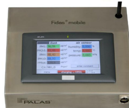
FIDAS mobile (Palas) PNC, size-distr. (32ch/decade) 0.2-18 \mu m PM 10 /4/2.5/1
