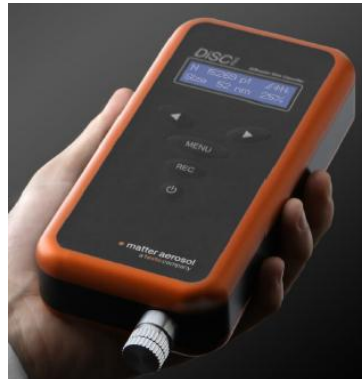
DiSCmini (Matter Engineering) PNC/LDSA(alveo.) 10-300 nm modal
